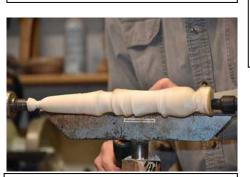
16. The last steps are to get the point final tapered, and to round off the top, removing both mounting points. Sanding will help keep splinters down when the stake is out in the weather.
