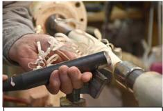
5. Cut a long taper to define the point on the bottom of the stake.
