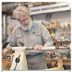
3. Mount the workpiece between centers on the lathe. Dick uses a cup center on each end and adds enough pressure so the tool can cut.
