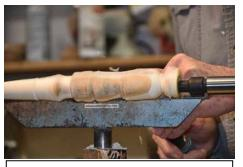
14. Re-mount the workpiece to a point 90 degrees from the 2nd center. This will allow you to turn away one side of the figure. Do the same cut on the opposite side, 180 degrees from the 3rd center.
