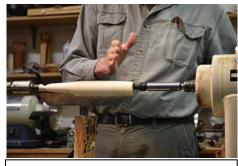
8. Re-mount the workpiece using the 2nd center.
