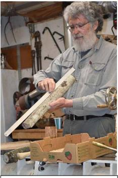
2. Using a straight edge, identify the axis of the stake.
