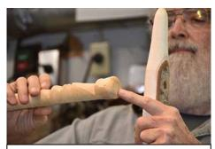
7. Roughly half-way between the real center and the back edge should be the 2nd center, raising the opposite side so you can define the facial features.
