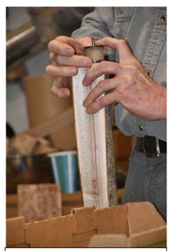
1. Dick starts with a piece of wood of the right length. He uses a pre-cut small cylinder to identify where the actual center of the stake will be.
