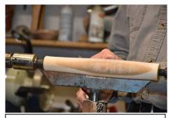
4. Start turning so the workpiece is partially round.
